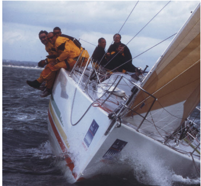
The hull and deck of this yacht were constructed from Kevlar and SYNTAC EPA epoxy resin with a pvc foam core using wet lay-up in a female mould and post cured at 45°C .
