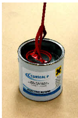
Mix thoroughly with a spiral mixer used in a cordless drill
