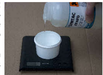
Digital kitchen scales are ideal for weighing out small amounts of material
