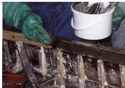
Cellulose fibres thicken epoxy resin to make an excellent gap filling adhesive.
