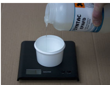
Digital kitchen scales are ideal for weighing out small amounts of material
