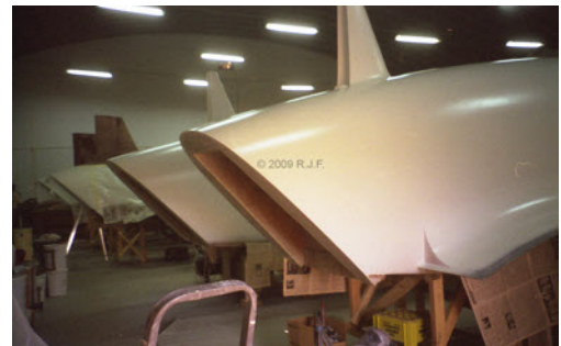
45' catamaran hulls being sprayed with Easy Fair HB.
